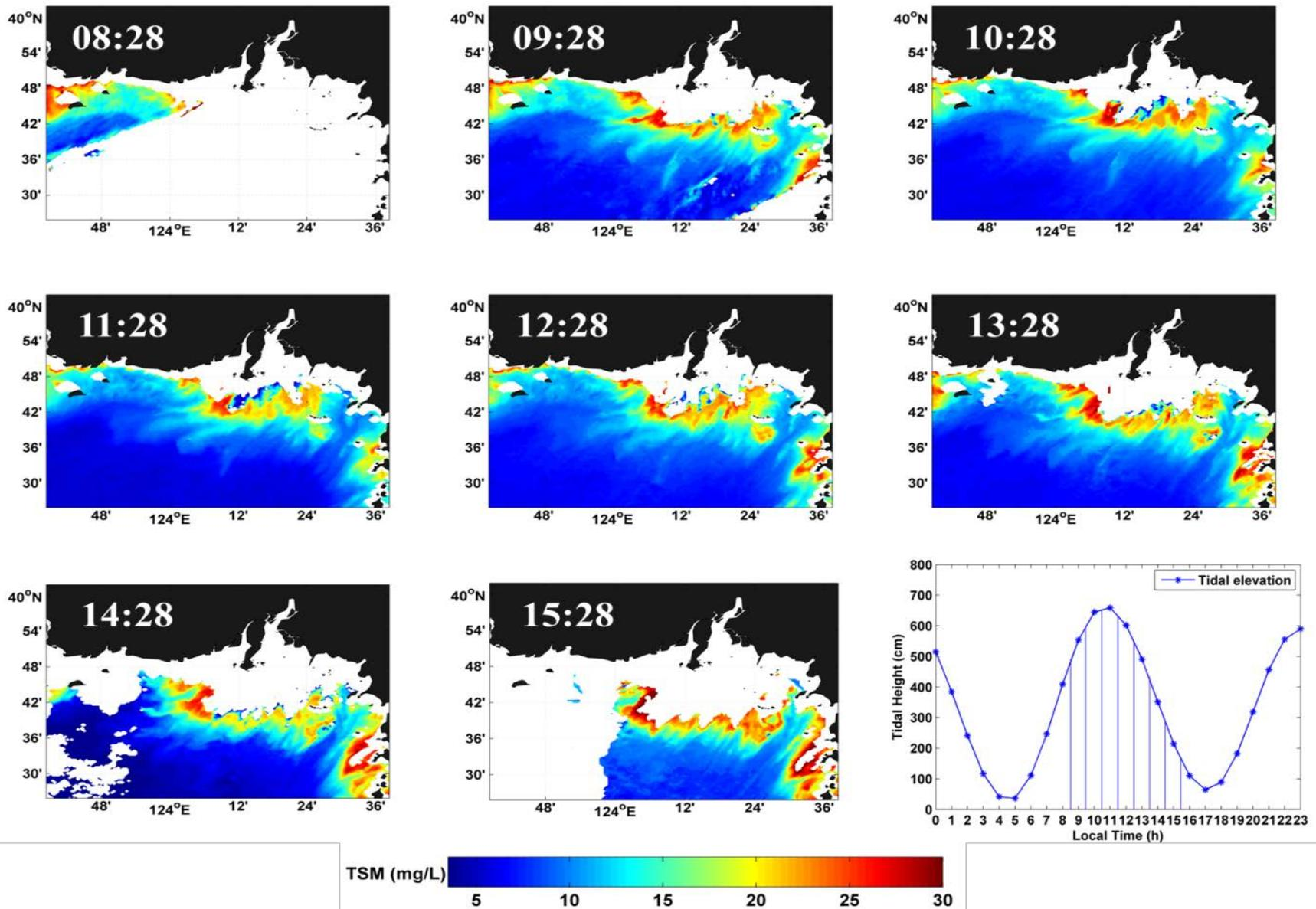
**Fig. 8.** Hourly maps of Total Suspended particulate Matter (TSM) from 08:28 to 15:28 (local time) in the Yalu River Estuary on 3 April 2014. The graph shows the hourly tide elevation on the same day.
