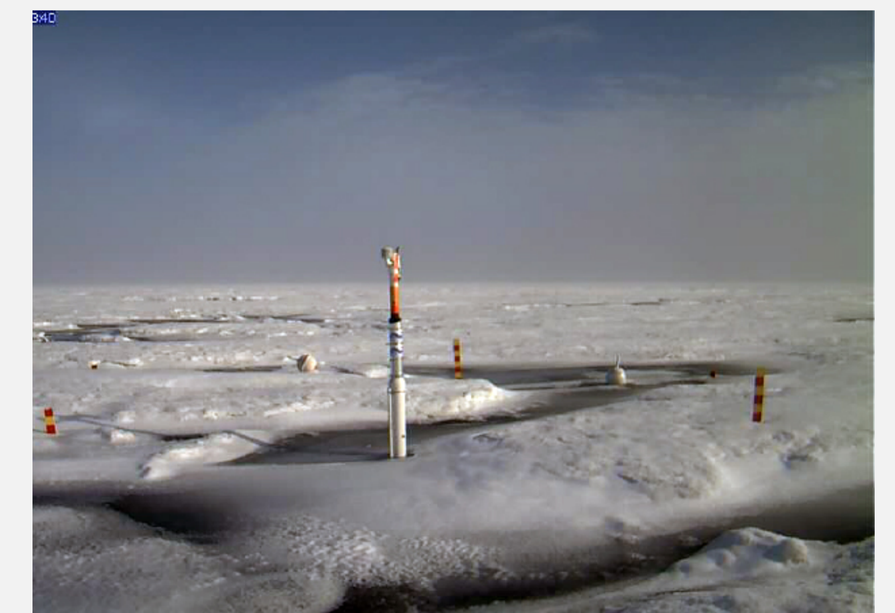
Fig. 4. Example of extreme conditions for ice buoys (round objects). Near-real time data can be screened using statistical tests, but the best option is to obtain the quality controlled post-deployment data from the buoy owner. The Arctic Buoy Program is working on ways to identify when ball buoys are in ice/ocean/air. Photo courtesy of U.S. Interagency Arctic Buoy Program.
