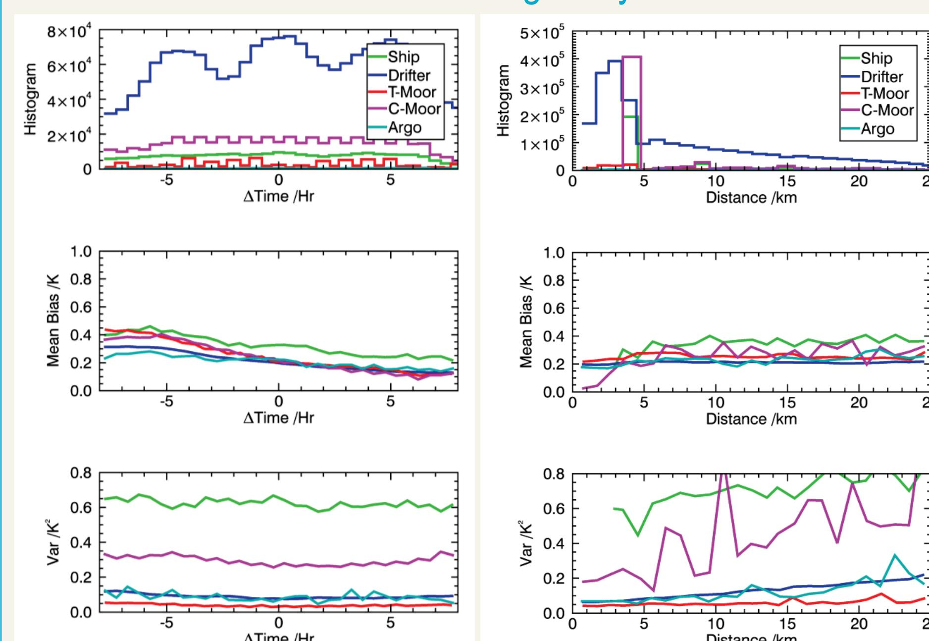
Figure 4: iQuam-AATSR match-up noise sensitivity over time (left) and space (right) separation. (Top, middle and bottom panels show histogram, mean bias and variance, of match-up  $\Delta SST$ , respectively)
