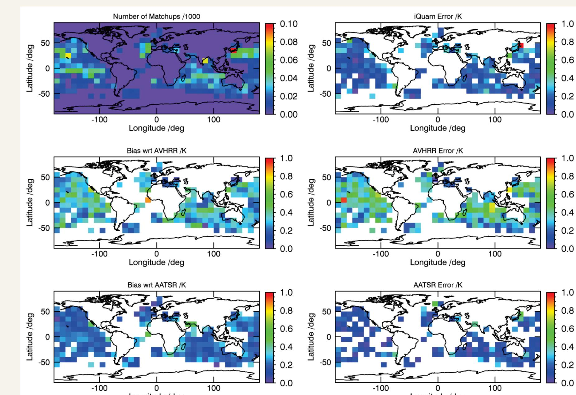
Figure 8: Geographic patterns of three-way error statistics of Argo-AVHRR-AATSR.
