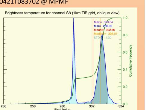
SLSTR-L1B-CV-270: Radiometric bias characterisation: Inter-satellite comparisons -MetopA/IASI/AVHRR with S3A/SLSTR
