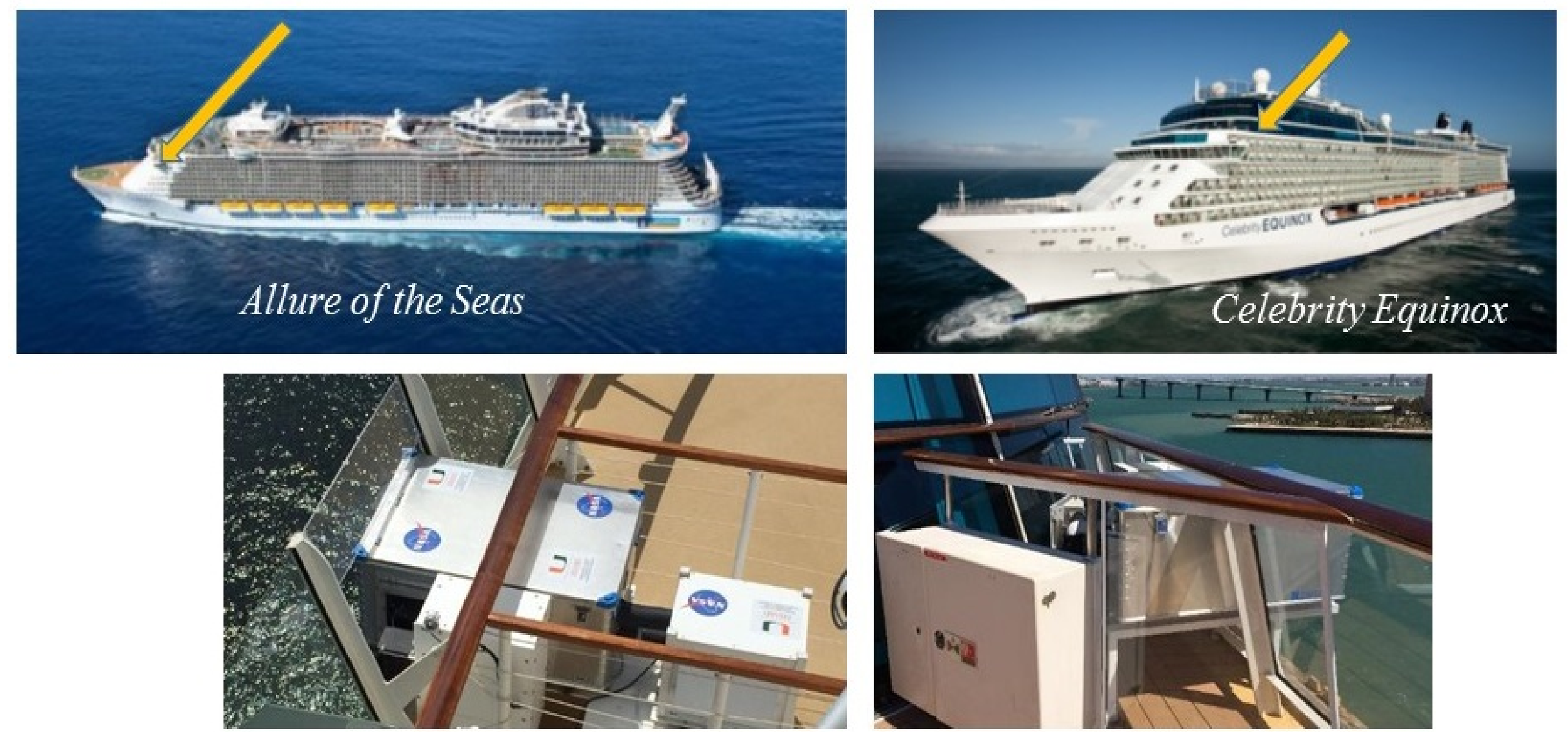
Installations of M-AERI Mk2 on cruise ships (yellow arrows). The instruments are inside hermetically sealed aluminum shipping crates, with the fore-optics on the sheltered, aft sides of the enclosures. The smaller boxes contain air-conditioning units to limit temperature and humidity variations in the instrument enclosures.
