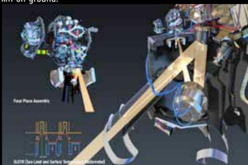
On the left image, the optical path inside the focal plane array (FPA) to the visible (yellow-multi-coloured path) and infrared (red path) detectors is shown. The flip-mirror assembly is to the bottom of the image shown in cutaway. This selects which optical path – from the nadir or oblique scan mirror – is directed into the FPA. On the right the path taken to inside the visible and shortwave infrared (purple path) detectors is revealed FPA.
