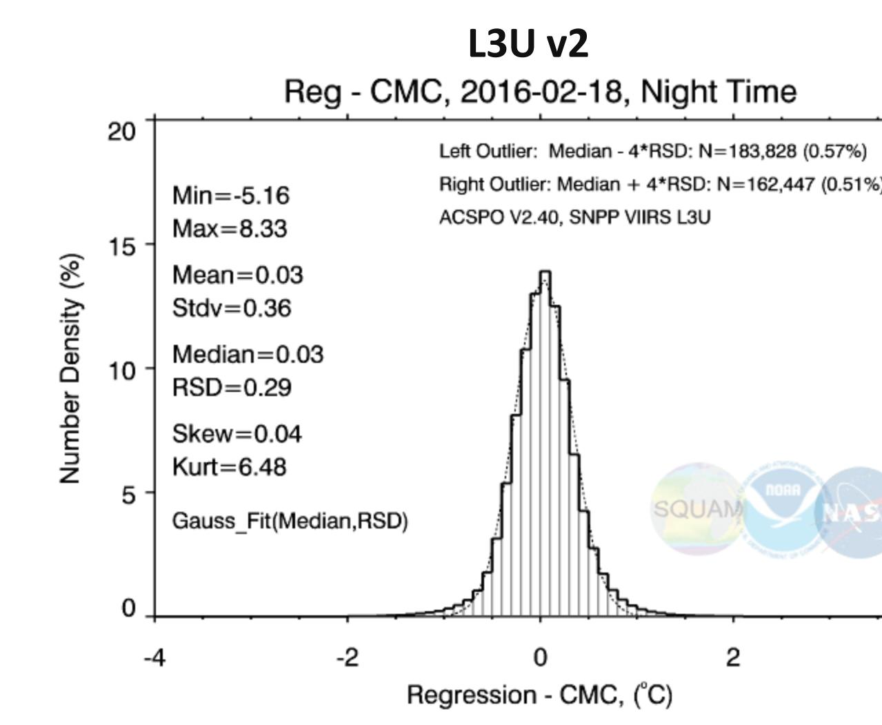
Fig. 6: Differences between nighttime L3U and L4 (CMC) for 2016-02-18.
