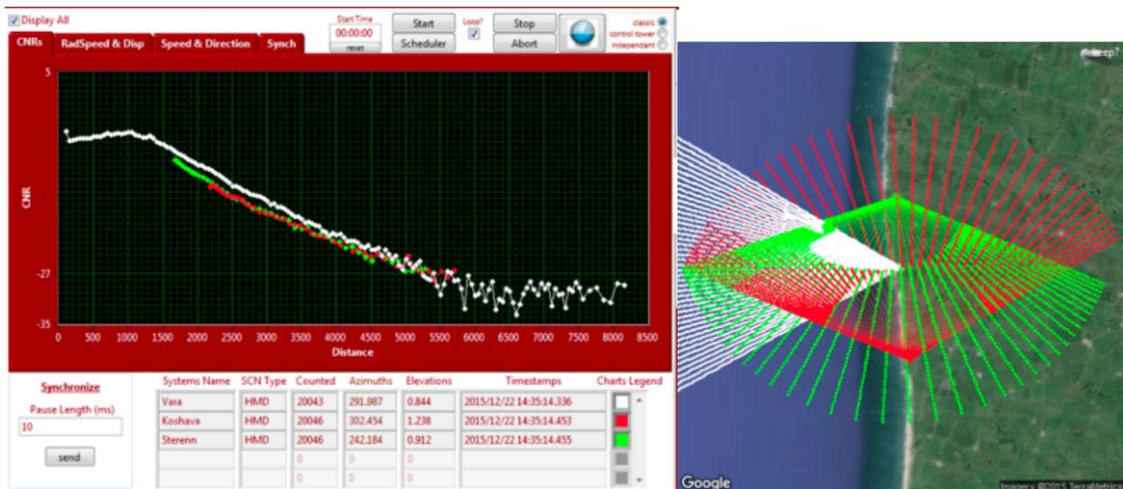
Figure: Carrier to Noise Ratio (CNR) as a function of distance (left) and scanning pattern (right).
