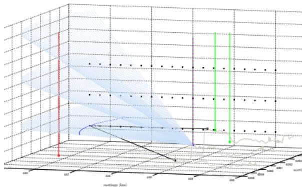
Figure: 3D overview of the measurements. Blue points: range gates from the scanning LIDAR, black points: dual Doppler, vertical lines: profiling LIDARS.
