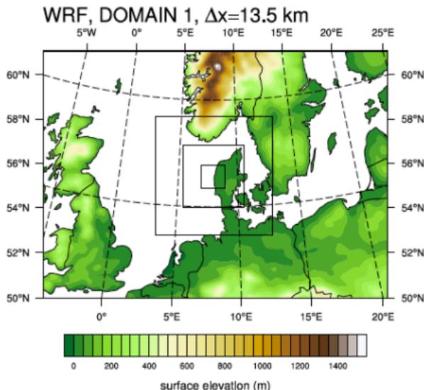
Figure: Domain configuration for the RUNE sensitivity simulations
