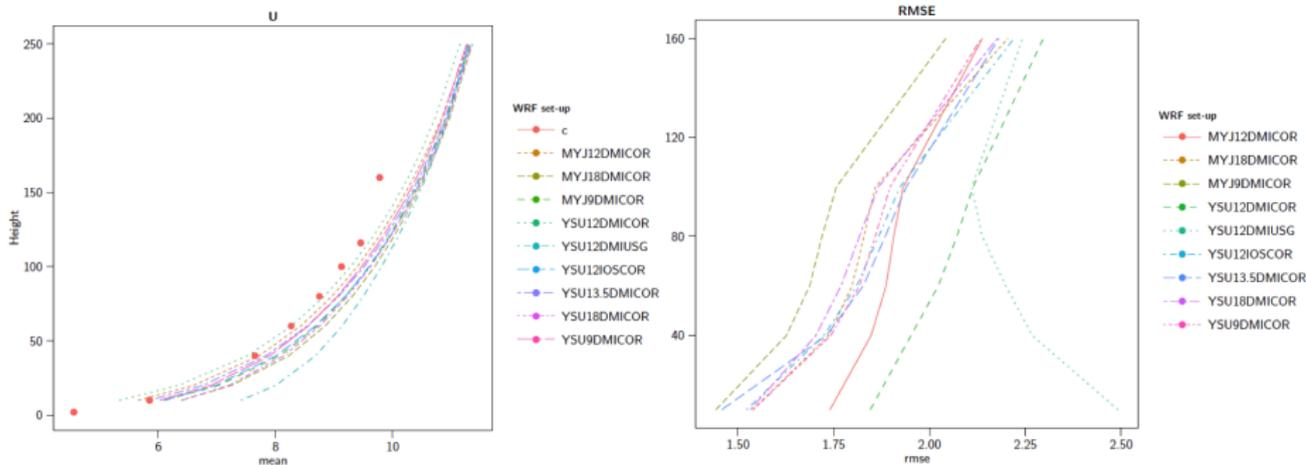
**Figure:** Mean wind speed profile from the cup anemometers (c) and different WRF set-ups, at Høvsøre. Right: RMSE of the wind speed profile between measurements and WRF simulations.
