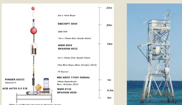
The left panel shows the ADCP-based current and wave monitoring system and the attached SBE39 temperature sensor. The right panel shows the AIMS FAIMMS station.
