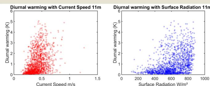
Data from the GBRPPS station (18.18°S 147.09° E), period: Oct 24 2012 to Mar 27 2017. The ADCP depth is 68 m and the SBE39 temperature is at 11 m depth. Left figure shows the relationship between the diurnal warming, defined as the temperature range in 24-hour periods, and the maximum current in the same intervals. Right figure shows the relationship between the diurnal warming and surface radiation.
