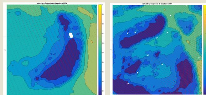
Arrows show flow velocity time 27.78 days, after the model has spun-up. The right panel shows a close-up of a reef system with northward currents at the top and southwestward current. Note that the visualization was performed by interpolating the model output on a regular structured before contouring. The contours are bathymetric depth.
