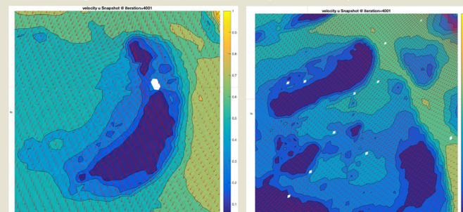
The flow velocity at time 34.85 days. The current flow is driven by tidal forcing. Initial results show that the tidal currents are strongest in shallower water, not supporting the "sticky water" hypothesis of Wolanski & Spagnol. (2000). Additional simulations are needed to resolve and understand the physical causes of the signals.
