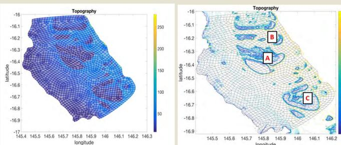
The left panel shows the full spectral element grid including the interior interpolation points. The right panel shows the 1596 elements partition of the domain. Locations of three positions at different depths in the model domain are shown.
