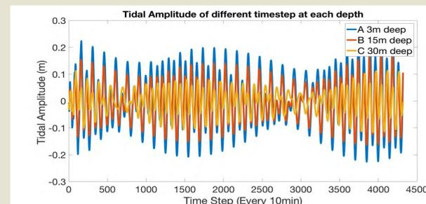
Time series of pressure fluctuations at three locations at model grid point at different depths, indicating larger amplitudes of the tidally induced variations in shallower water.
