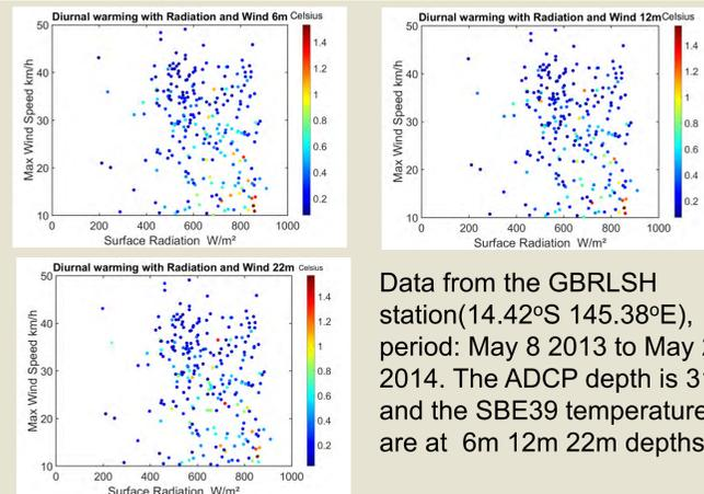
Data from the GBRLSH station(14.42°S 145.38°E), period: May 8 2013 to May 21 2014. The ADCP depth is 31m and the SBE39 temperatures are at 6m 12m 22m depths.
