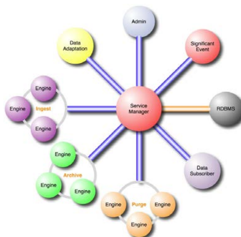
Figure 3. The top-level DMAS system architecture view.
