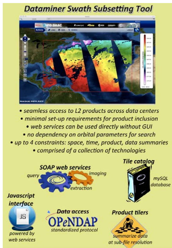
Figure 2. The features and components of the NAIAD/Dataminer system.
